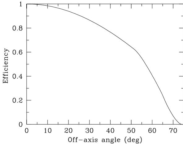
**Fig. 1.** Detector efficiency as a function of source off-axis angle (same for both WATCH energy bands)
