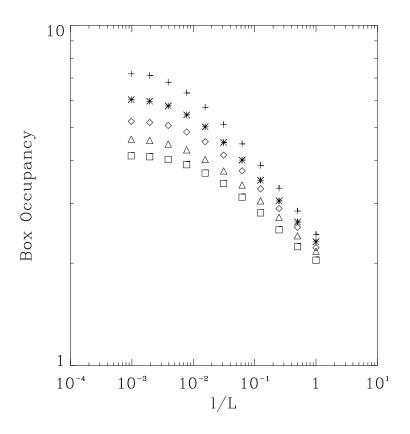
Figure 3: Normalized box occupancy A as a function of length scale, normalized to the integral scale L. The symbols represent, from top to bottom: z = 2, 2.5, 3, 3.5, 4.
