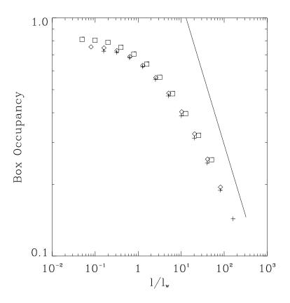
Figure 5: Rescaled box occupancy  $Au_0/u'$  in convective turbulence (eddy-velocity scaling exponent  $\eta = 5/3$ ) as a function of length scale, normalized to the cutoff scale  $l_w$ . The correspondence between symbols and z values is as in figure 3. The line corresponds to a linear decline with a slope of -3/5.
