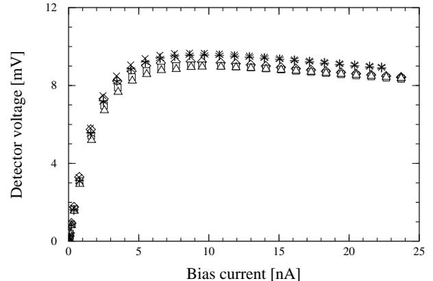
Fig. 7.— Plot of six bolometer I-V curves. The non-ohmic behavior, shown in the roll-over at  $\sim 5$  nA, is caused by electrical self-heating in the detector. The excellent matching of the detectors is evident, especially at high bias. The six detectors cluster into two rows of three in which the voltages are virtually identical.
