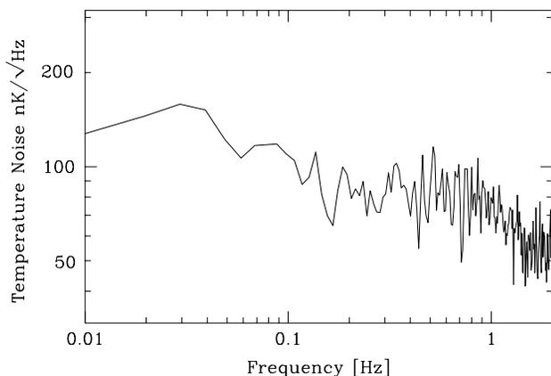
Fig. 12.— Measured temperature noise of the 300 mK cold stage monitor thermistor.
