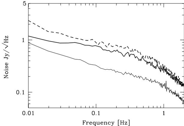
Fig. 15.— SuZIE system noise for the difference between 2 detectors separated by  $4.3'$ . The solid line corresponds to the 142 GHz band, the heavy line the 217 GHz band, and the dashed line the 268 GHz band. The data for three spectral bands are calibrated in terms of Janskys by observations of planets.
