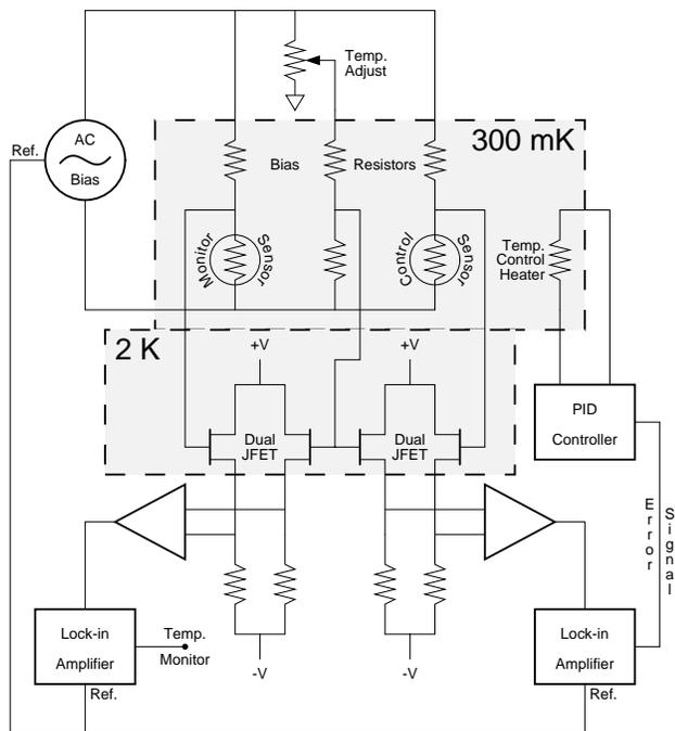
Fig. 11.— The SuZIE temperature control electronics. Two thermometers mounted on the optics block are differenced against fixed resistors. A variable bias resistor allows adjustment of the temperature set point. The output from one bridge is used as the error signal for a proportional-integral-differential (PID) controller, which closes the control loop using a heater on the optics block. The other bridge is monitored to determine the temperature stability.
