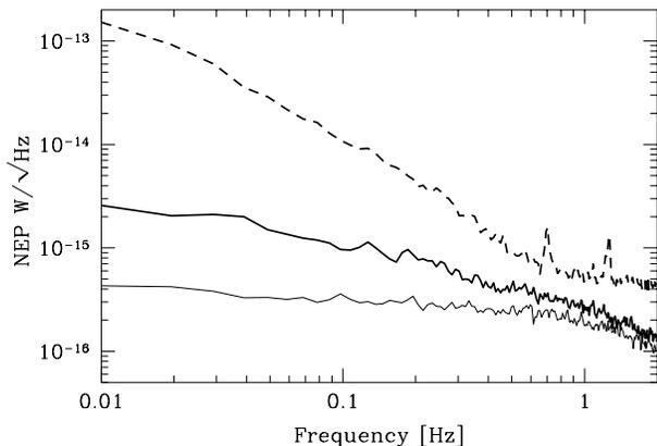
Fig. 10.— SuZIE system noise for a detector difference as measured in the laboratory with an optical blank in place of the Lyot stop (solid line). Also shown is the noise for the system at the telescope in the 217 GHz configuration, for both a single detector (dashed heavy line) and for a detector difference (heavy line). The results are calibrated in terms of NEP using the measured electrical responsivity of the detectors.
