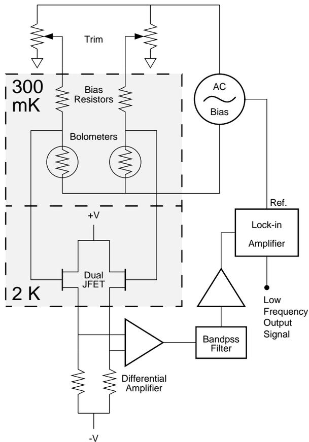
Fig. 8.— AC-bridge readout for bolometers. The bias resistors are large compared to the trim resistors, which are needed to compensate for mismatches in the bolometer responsivities. The initial amplification stage is mounted on the  $^4\text{He}$  cold-plate to reduce the amount of high impedance wiring. In the SuZIE experiment, both bolometers are exposed to the sky, and the output is proportional to the differential sky brightness.
