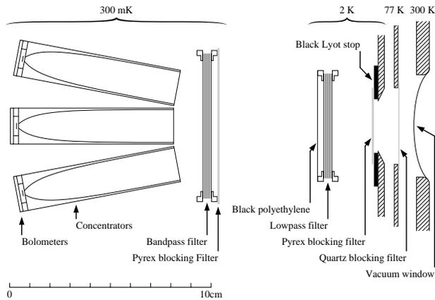
Fig. 4.— Configuration of the filters and optics inside the  $L^4\text{He}$  cryostat.
