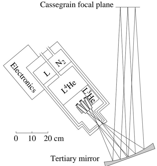
Fig. 3.— Coupling of the SuZIE receiver to the CSO using a fixed tertiary mirror. The cryostat can be rotated around its optical axis to keep the array aligned with the direction of sky drift.
