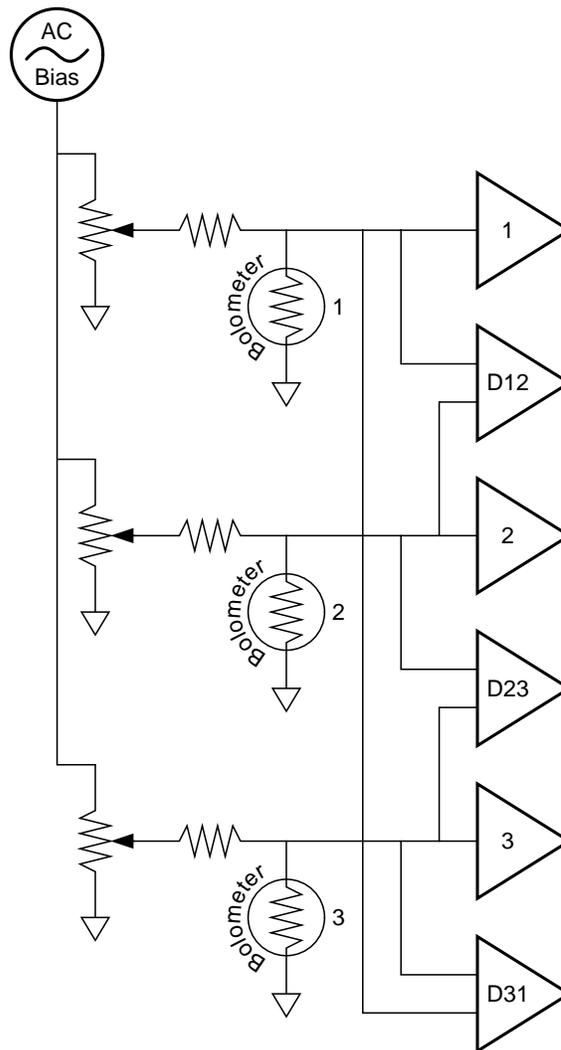
Fig. 9.— One row of the SuZIE readout electronics. Each row has a single bias, three difference channels, and three absolute channels.
