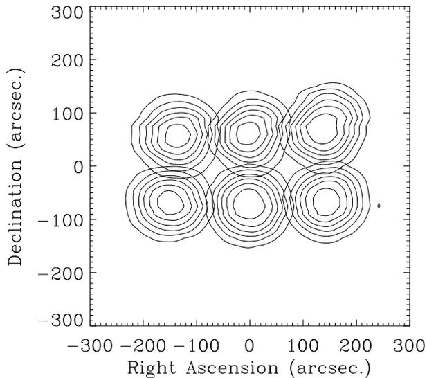
Fig. 13.— Map of bolometer single channels at 142 GHz constructed from drift scans across Jupiter spaced by  $15''$  in declination. Contours correspond to 0.9, 0.75, 0.6, 0.45, 0.3 and 0.15 of maximum. The large size of Jupiter ( $\sim 40''$ ) broadens the beams slightly.
