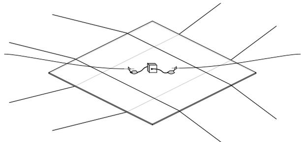
Fig. 6.— A composite bolometer used in the SuZIE instrument. The thermistor with wedge-bonded gold leads is secured to the sapphire substrate with two blobs of epoxy. The NbTi electrical leads have copper-clad ends, which are soldered to the gold wires. The substrate is suspended by four nylon threads.
