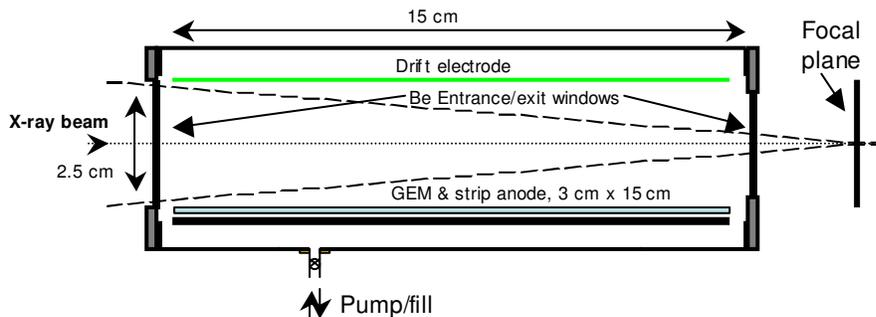
Figure 6: The TPC polarimeter concept. The design allows simultaneous polarization and spectroscopy observations.
