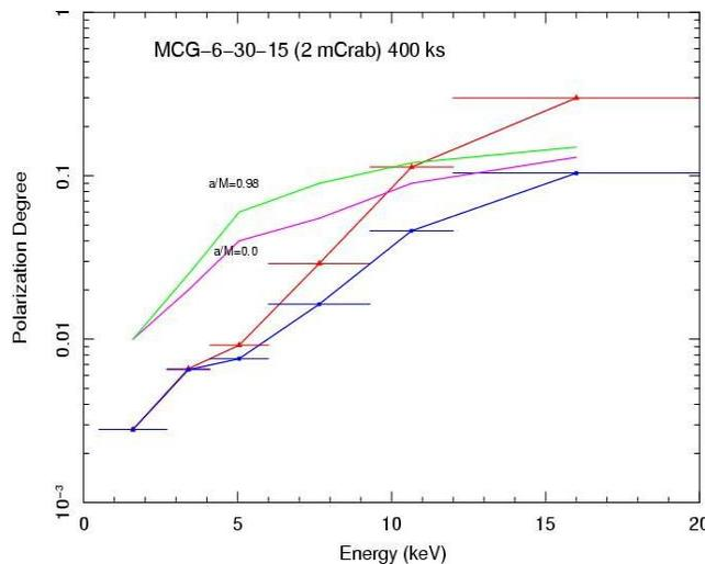
Figure 3. Polarization of an AGN with reflection from a disk source which is on axis a distance of  $2\text{GM}/c^2$  above the plane. The bars show the polarization detection limits for the energy range of the single Ne/DME detector (red) and the two detector, Ne/dimethyl ether and Ar, combination (blue). The green and magenta curves are for illumination of the disk by an unpolarized coronal source (See text).
