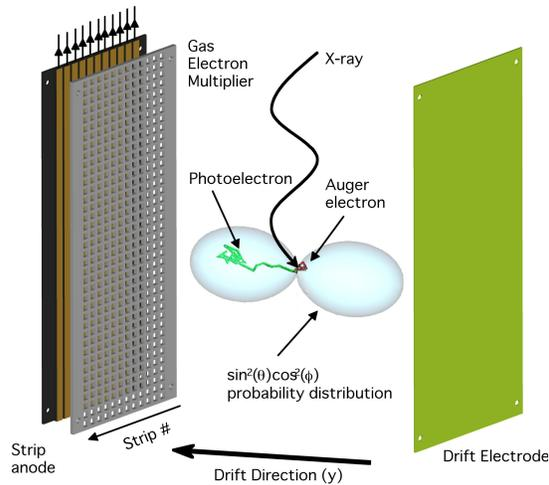
Figure 4a: The time projection polarimeter uses a simple strip readout, left, to form pixelized images of photoelectron tracks.
