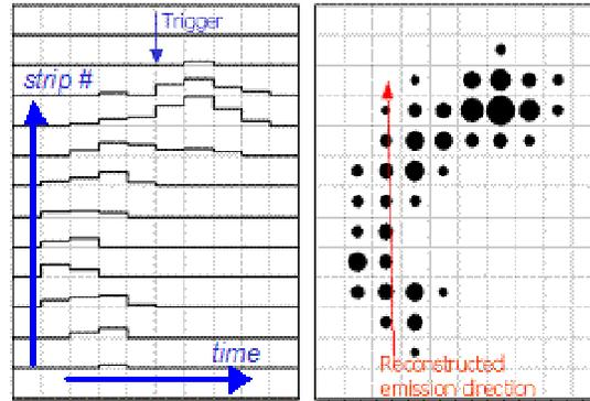
Figure 4b. The digitized wave forms are interpreted as the density of charge along the photoelectron track. In this image, the horizontal axis is time and the vertical axis is readout strip. The size of the dot is proportional to charge.
