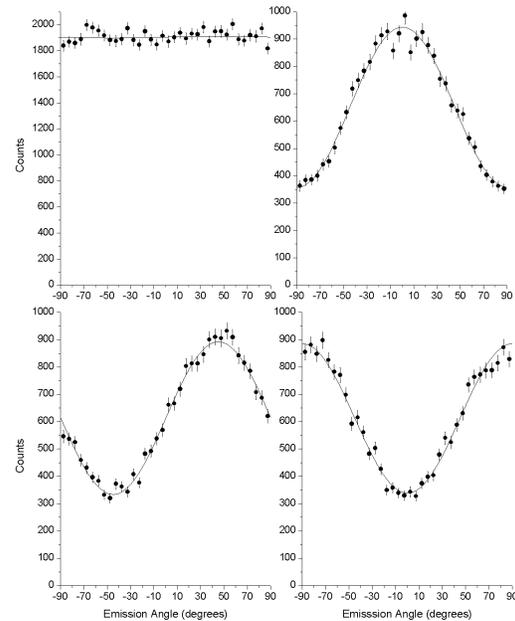
Figure 2: The modulation response of Goddard's demonstration polarimeter to unpolarized 5.9 keV Fe-55 X-rays (upper left) and 100% polarized X-rays with the detector in three orientations with respect to the beam. The measured polarization of the Fe-55 X-rays is  $0.49 \pm 0.54\%$ . The other three measurements are consistent with  $45 \pm 1.1\%$  modulation. The detector was filled with 460 Torr of a 50/50 Ne/dimethyl ether mixture.
