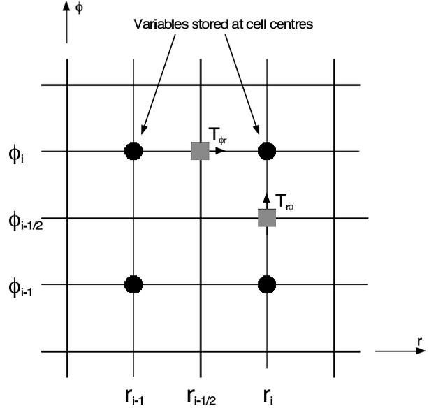
**Figure 1.** Storage of variables in FLASH. All variables are stored at cell centres, located at  $\{(r_i, \phi_j), (r_{i+1}, \phi_j) \dots\}$ . The cell faces are located at the ‘half’ positions. We require the components of the stress tensor to be centred on the cell faces
