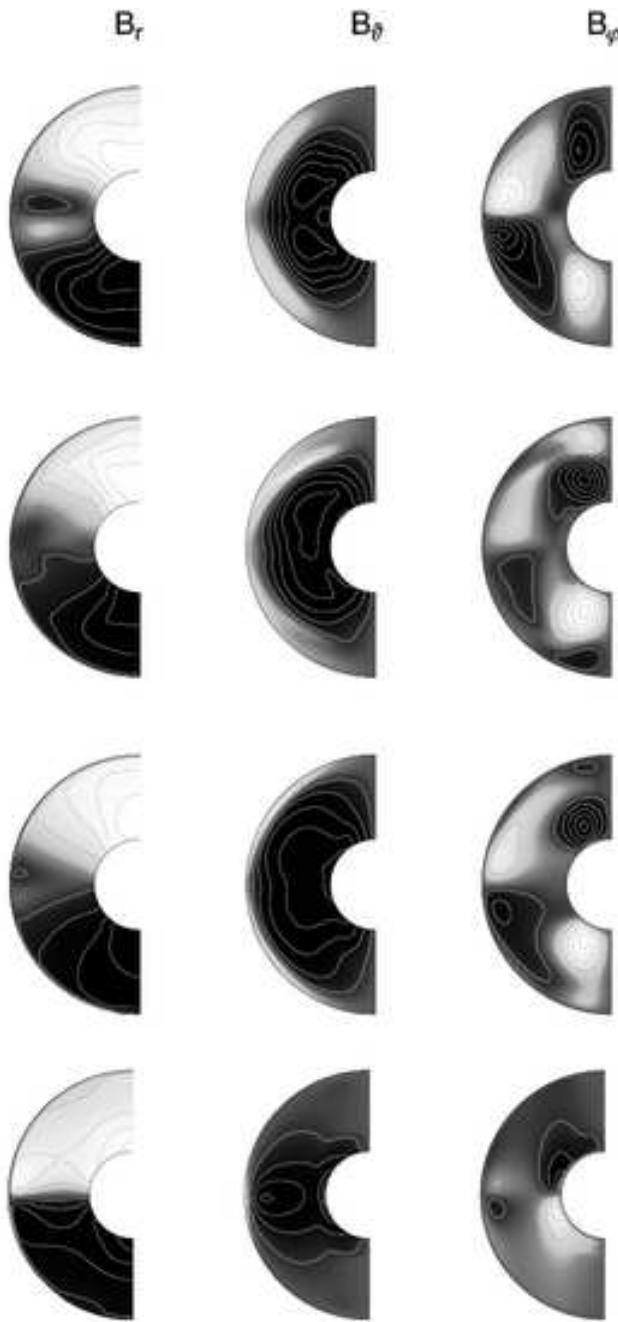
Figure 10. Comparison between numerical simulations and mean-field calculations in the example of the geodynamo: azimuthally averaged magnetic field components resulting from a direct numerical simulation (first row), results as given by mean-field modelling with coefficients derived by approach I (second row), mean-field calculation with coefficients in SOCA (approach I with \mathbf{G} = \mathbf{0} , third row), and with coefficients for isotropic turbulence (last row). Different from the solution of the direct numerical calculation which is stationary, all mean-field solutions decay exponentially with decay rates \lambda = 3.5 \eta/D^2 (second row), \lambda = 6.5 \eta/D^2 (third row), and \lambda \approx 75 \eta/D^2 (last row).
