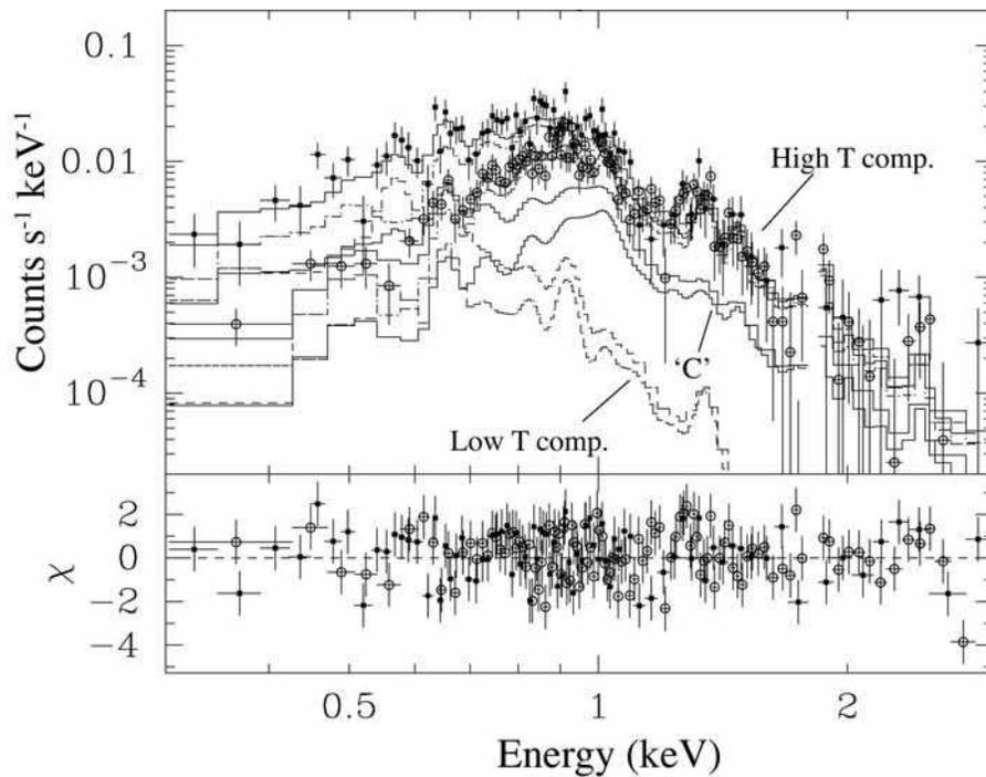
**Fig. 4.** The simple background-subtracted XIS spectra of the Cap are shown with the best fit 2vMEKAL model spectra. Black squares indicate the BI (XIS1) spectrum. The open circles show the combined spectrum of the three FI (XIS0,2,3) with the normalization for one FI sensor.
