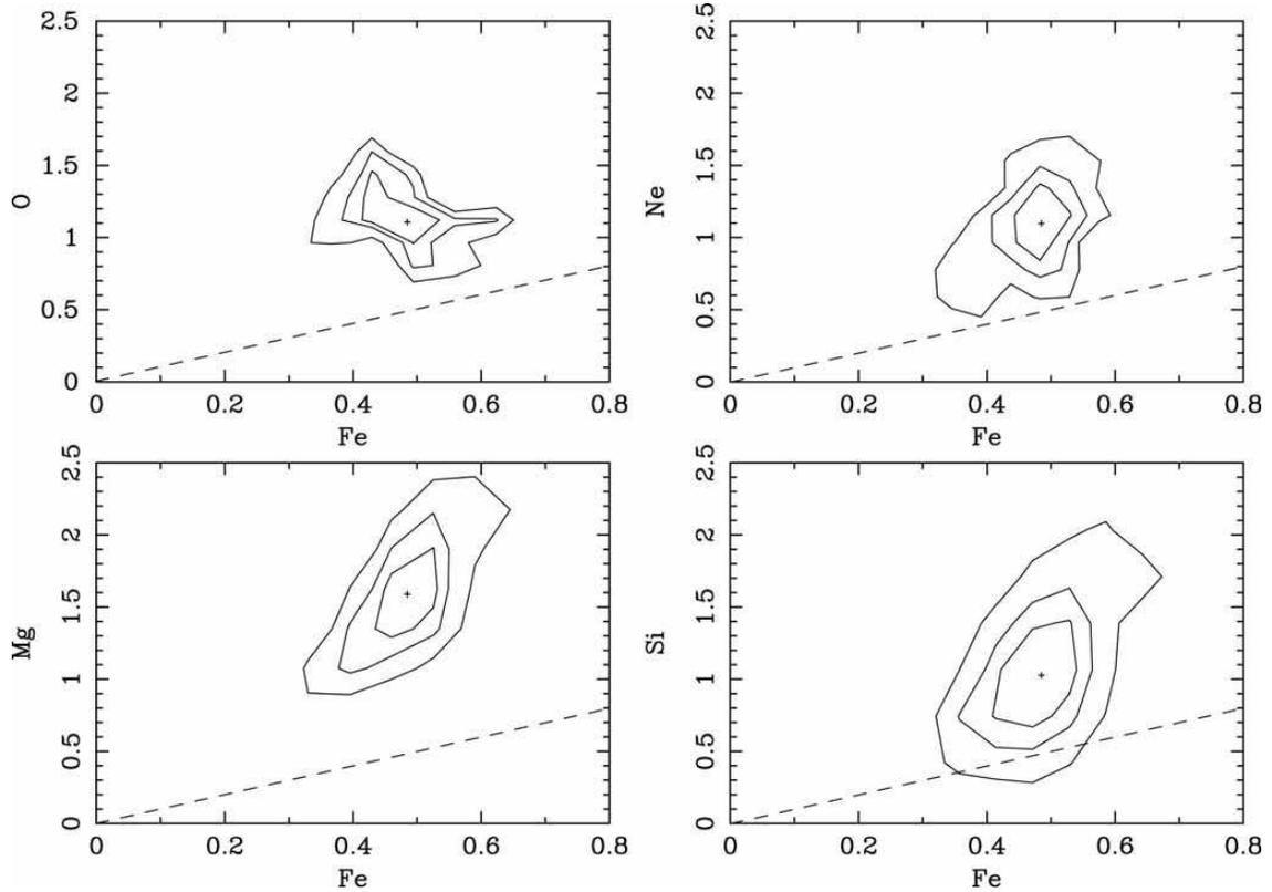
**Fig. 9.** The confidence contours for the O, Ne, Mg and Si abundances relative to the Fe abundance, obtained from the fits using the 2vMEKAL model. The contours are given at confidence levels of 68%, 90% and 99%. The dashed lines show the solar abundance ratio between the metals.
