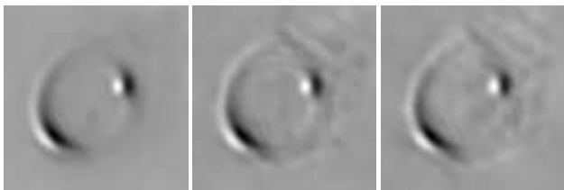
Figure 12. Differences between the beam-convolved true lens image and the CLEAN reconstructions. Left: the 3 hour observation with no errors. Centre: The 1 hour observation with no errors. Right: A 1 hour image with gain/phase errors. In each case, the peak of the difference is approximately 10% of the peak in the image, or \sim 20 \text{ mJy} .
