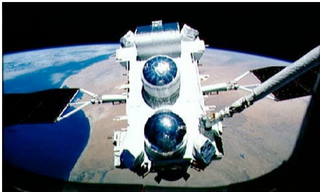
Fig. G1. The Compton Gamma-Ray Observatory (CGRO) as it was being deployed from the space shuttle Atlantis (STS-37). COMPTEL is the instrument located in the center of this S/C, between the solar panel mounts.
