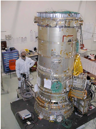
Fig. G6. INTEGRAL/SPI BGO shield [110], comparable in size to that of ACT.
