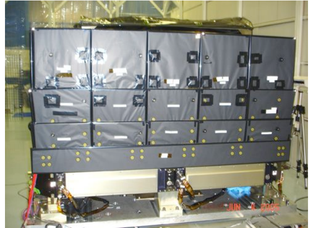
Fig. G7. GLAST ACD shield [74], comparable in size and design to that required by ACT.
