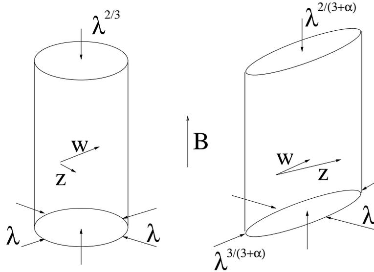
Fig. 1.— A sketch of the shapes of turbulent fluctuations, “eddies,” in the Goldreich-Sridhar picture (left), and in our picture (right). The large-scale magnetic field is denoted by  $\mathbf{B}$ . As the turbulent cascade proceeds toward the smallest, dissipative scales,  $\lambda \rightarrow 0$ , the Goldreich-Sridhar “eddy” assumes the shape of a filament, while the “eddy” predicted in our model turns into a current sheet.
