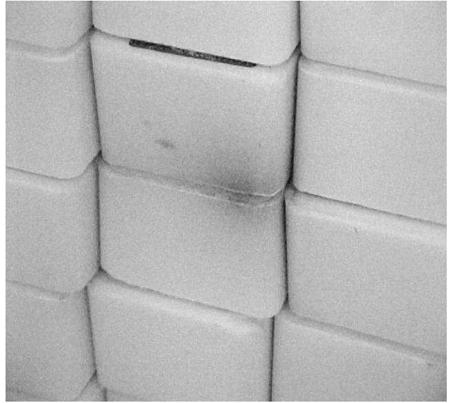
FIG. 5: The exit point of the beam in the downstream wall of the salt target, outlined by discoloration of the salt produced by beam and showing in cross section at the exit surface. Even at this location of order 15 radiation lengths along the shower, the shower core is still only several cm across (the salt blocks are 6 by 10 cm here in cross section).
