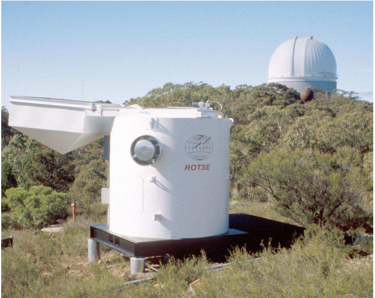
Fig. 3.— The ROTSE-III telescope enclosure at the Siding Springs Observatory near Coonabarabran, Australia with the hatch cover fully open. The telescope optics have not yet been installed. The 4-meter Anglo-Australian telescope is in the background.
