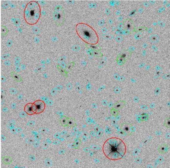
FIG. 10.— Combined F555W WF2 image. North is up and East is left. The ellipses indicate the region extending to  $4\times$  the isophotal detection radius, as discussed in §10. Red ellipses mark galaxies with  $V_{555} \lesssim 23$  AB mag; green ellipses,  $23 < V_{555} \lesssim 25$  AB mag; and blue ellipses,  $25 < V_{555} \lesssim 28.5$  AB mag. All sources in the catalog are shown. The completeness limit is  $V_{555} \sim 27.5$ .
