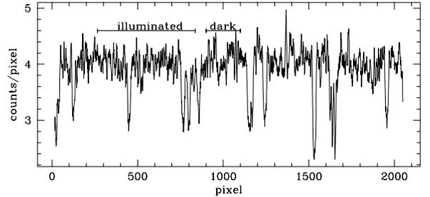
FIG. 15.— Average of 25 FOS dark exposures (1300 sec), demonstrating the stability of the pixel-to-pixel structure of the dark signal. Strong features appear where diodes have been turned off due to poor performance. Sub–stepping along the diodes allows complete spectral coverage over these dead diodes.
