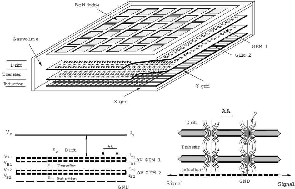
Figure 3. Schematic of detector with two GEM multiplication stages.
