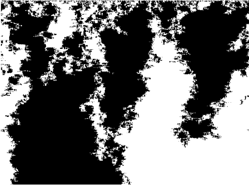
Figure D.15: Computer simulation of a one-round cellular game, the Cloud Process, on a ring of 640 cells. The table for this game is: G(BBB) = G(WWW) = 0.27 , G(BBW) = G(BWB) = G(BWW) = G(WBB) = G(WBW) = G(WWB) = 0.53 . Program cloud.pas , random seed 118950941. Initial conditions were chosen with the aid of a pseudorandom number generator.
