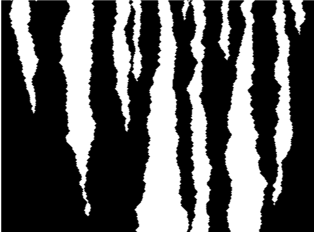
Figure D.22: The annihilating particle model, on a ring of 640 cells, which initially contains 28 particles. Program apm.pas , seed 269093635. Each particle executes a symmetric random walk, having a 50% probability of going either left or right in each generation.
