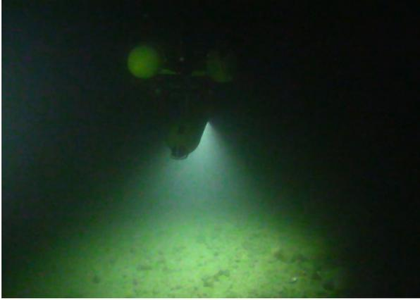
Figure 2. Autonomous underwater vehicle in 100m depth in coastal waters. Note the illumination pattern at the seafloor as well as the scattering (the light cone) in the water.
