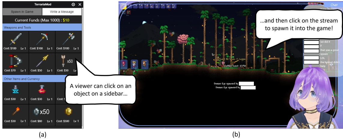
Figure 1: VIBES allows audience members of a livestream to spatially interact directly with the streamed application through mouse events on the video player. In this example, viewers can spawn items into a game by first clicking on the item on the Twitch extension (a) and then clicking on the desired spawn location on the streamed game (b).
