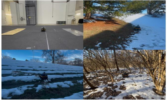
Fig. 4: Real-world experiment environments with various surfaces and physical properties. The vehicle’s left front axle was broken as an anomalous situation, whereas the additional rock posed challenging inertia force.
