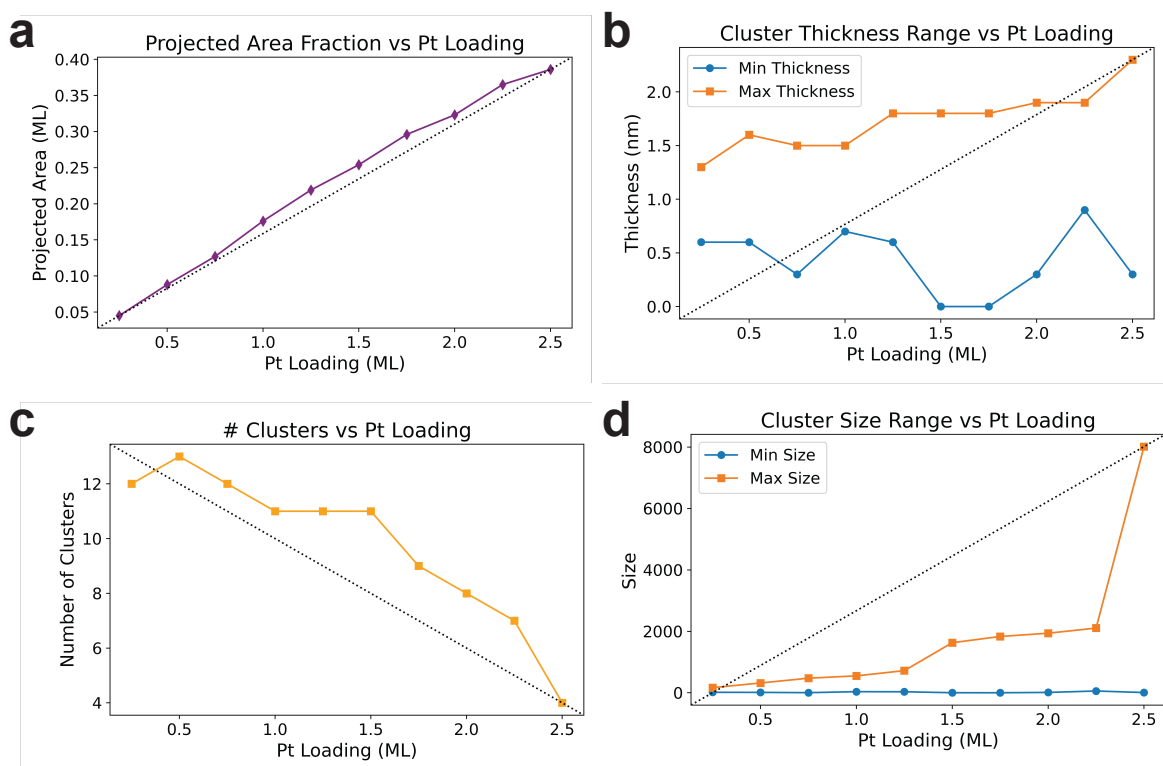
Figure S2: Cluster Properties versus Pt Loading. a Projected area fraction (Pt clusters' projected area divided by graphene area). b Minimum and maximum cluster thickness versus Pt loading. c Number of clusters formed at different Pt loadings on graphene. d Minimum and maximum cluster size versus Pt loading. The same data are reported in Table S1.
