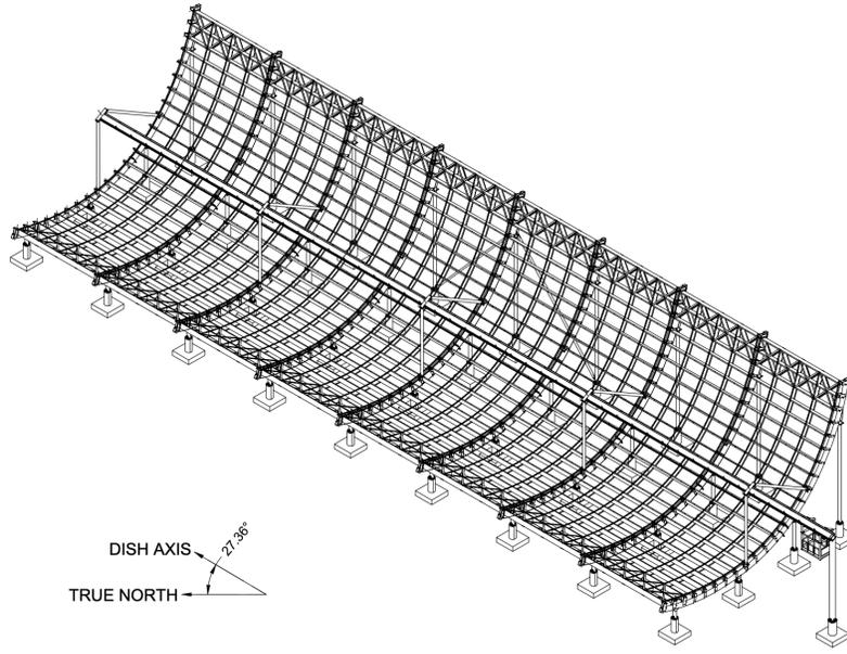
**Figure 3.** Isometric view of the structural drawings for the GBO station. Due to its Eastward location, the GBO station requires a substantial axial roll and a rotation from local North (in the plane of the ground) so as to approximately match its field of view to CHIME’s along the meridian at DRAO. Image credit: Sightline Engineering.
