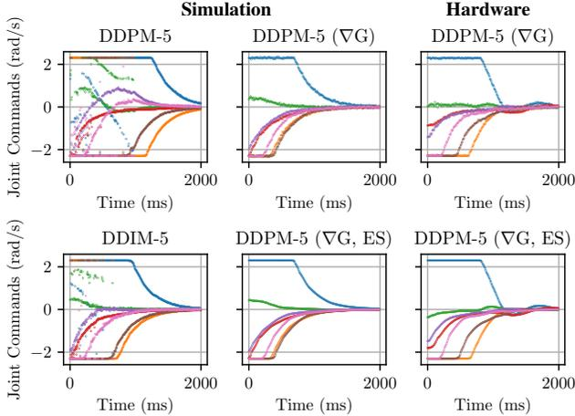
Fig. 4. Exemplary closed-loop joint commands of vanilla diffusion models in simulation (left), the DDPM with gradient guidance ( $\nabla G$ ) in simulation (center top) and hardware (right top), the proposed DDPM with five steps,  $\nabla G$ , and early stopping (ES) in simulation (center bottom) and hardware (right bottom).  $\nabla G$  ensures consistent modes necessary for hardware deployment, while ES smooths the commands.
