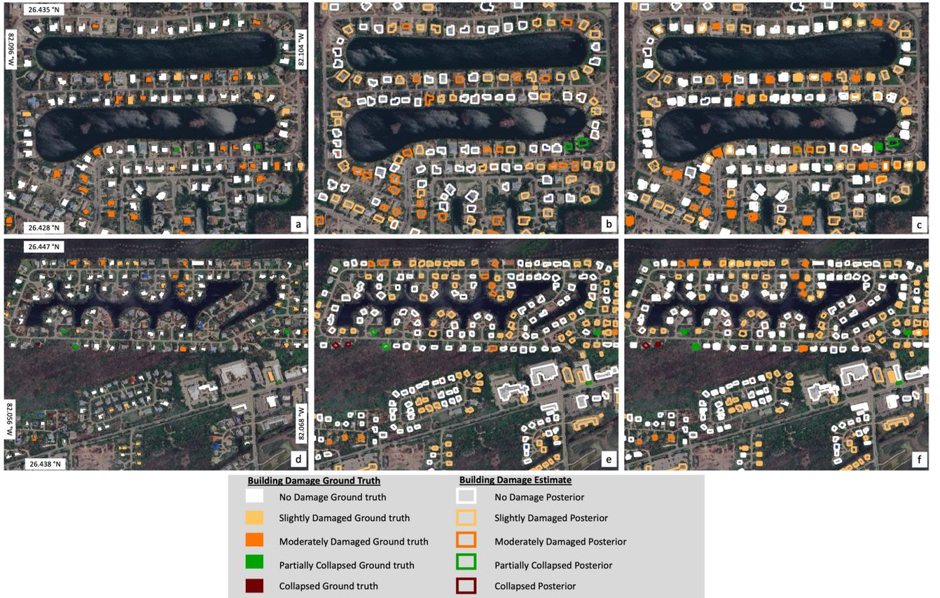
Figure 4: **Estimated building damage probability maps for Hurricane Ian case study in Lee County, Florida.** Figures (a)–(c) present the building damage ground truth, building damage estimation, and their overlay for the region from 82.096°W to 82.104°W and 26.238°N to 26.435°N. Figures (d)–(f) present the corresponding views for the region from 82.056°W to 82.068°W and 26.438°N to 26.447°N. Colors in the legend indicate building damage levels.
