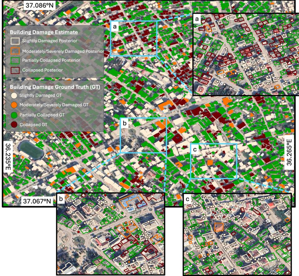
Figure 3: **Estimated building damage probability maps in Osmaniye, Turkey.** Figures (a)–(c) present the building damage estimates with ground truth information. The legend colors represent the building damage levels, as indicated.
