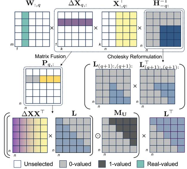
Figure 3. Computing paradigm of the second term for residual output error in  $q = 2$  iteration. The inverse Hessian matrix is factorized by Cholesky Decomposition, furthermore,  $\Delta \mathbf{X}_{q,:} \mathbf{X}_{:,q}^\top \mathbf{H}_{-q}^{-1}$  is fused to the  $q$ -th row of matrix  $\mathbf{P}$ , which can be computed in parallel. Dimensions are in the bottom left corner of each matrix.
