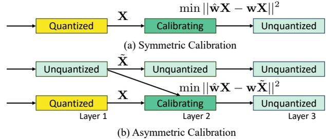
Figure 1. Calibration pipeline in the symmetric way (GPTQ) and the asymmetric way (GPTQv2).
