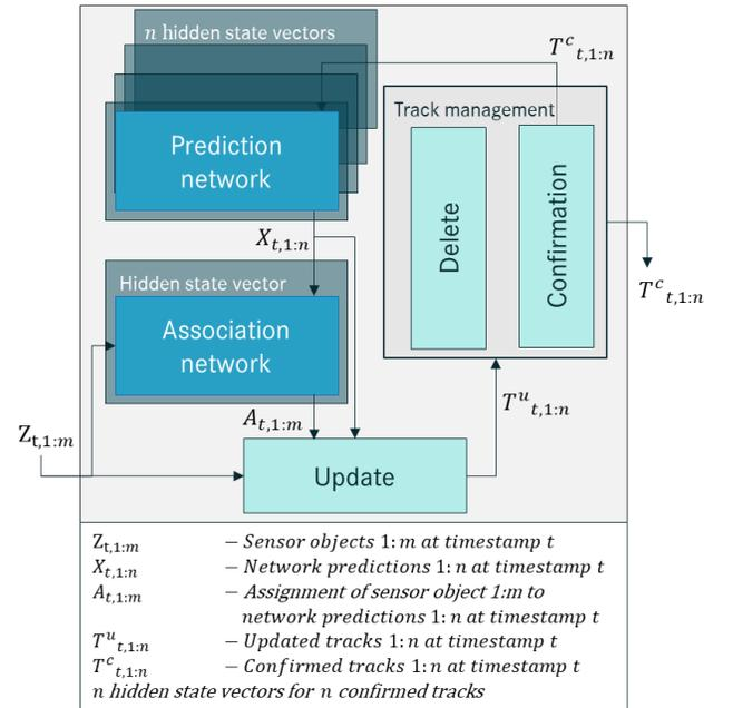
**Fig. 1:** This schematic representation shows the integration of two NNs (highlighted in dark blue) within a TbD framework. The "Association network" can be implemented using either SANT or MANTA. It works in tandem with the prediction network SPENT, which takes tracked objects  $T^c_{t,1:n}$  and predicts them to the next timestamp as  $X_{t,1:n}$ . The predicted objects are then associated with sensor observations  $Z_{t,1:m}$  by SANT or MANTA.
