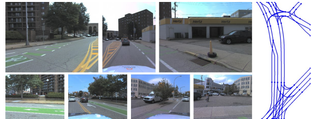
Fig. 1. Illustration of lane topology reasoning for high-definition (HD) mapping, adapted from OpenLane-V2 [5]. This example demonstrates the transformation from multi-perspective onboard camera images to a comprehensive bird's-eye view (BEV) lane topology representation.
