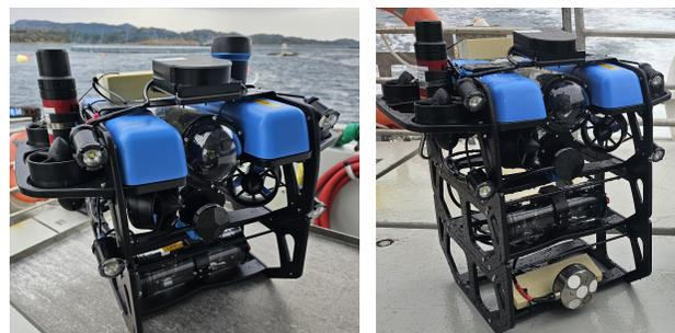
(a) ROV with sensor configuration 1. (b) ROV with sensor configuration 2.
