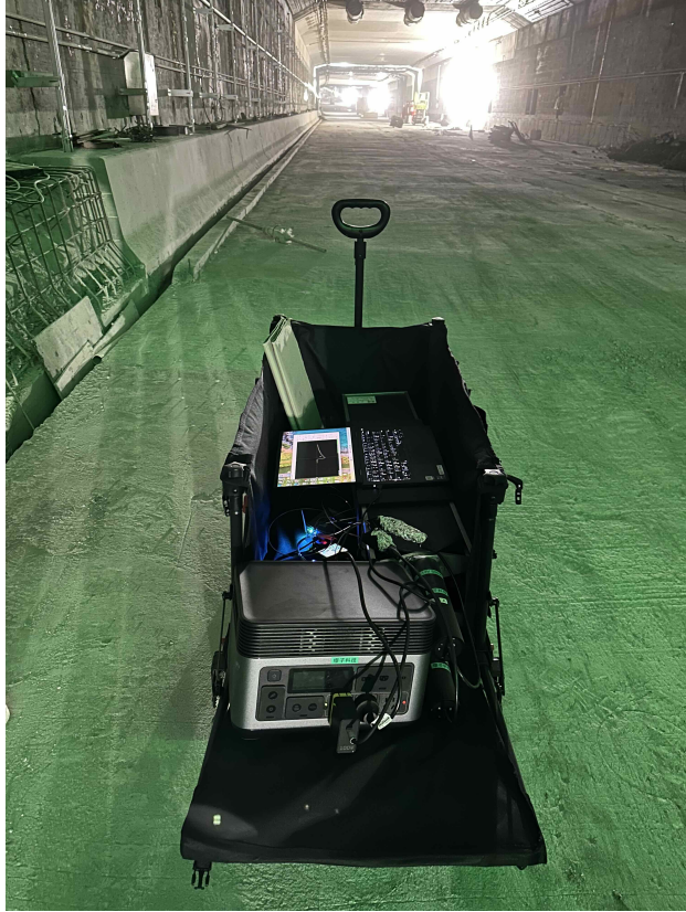
FIG. 6. A photograph of the muon detection system measuring muon flux at a location during the muon flux spatial scan campaign in the Shanghai Outer Ring Tunnel.
