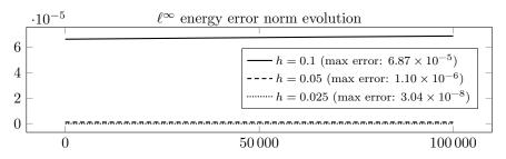
Figure 2: Over 100000 periods of motion, the  $\ell^{\infty}$  energy error growth rate is of:  $2.50 \times 10^{-11}$  when h = 0.1,  $5.45 \times 10^{-14}$  when h = 0.05, and  $1.35 \times 10^{-13}$  when h = 0.025.
