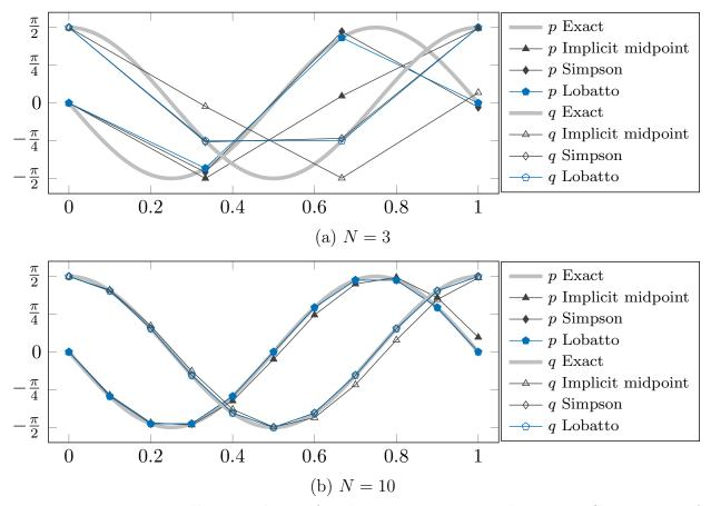
Figure 1: Harmonic oscillator evolution for the momentum p and state q. Comparison of the Lobatto symplectic scheme against the exact solution for (a) N = 3 meshes, and (b) N = 10 meshes. Lobatto's solutions are very close to the exact ones for as little as 3 meshes per oscillation period. Note that the momentum data have been rescaled.
