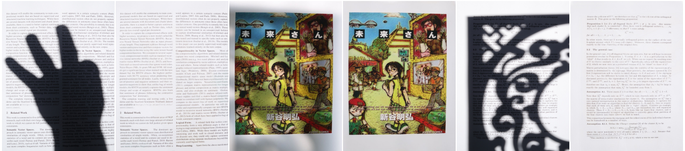
Fig. 1: Three sets of document shadow images and their corresponding shadow-free results obtained using our method are presented. From left to right, each set includes the shadowed image, followed by the image processed with our method, with the three sets displayed sequentially. Our method is capable of handling document shadow images from various scenarios, while preserving the text, patterns, tonal details, and other features that are covered by shadows in the original images as much as possible.
