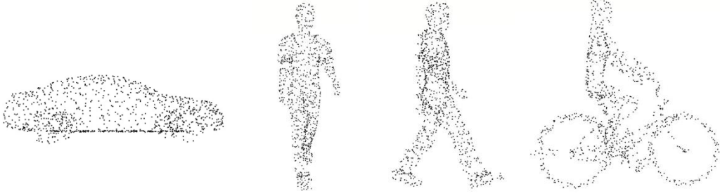
Fig. 2. Illustration of point cloud templates, where the pedestrian template is presented in its front and side views.
