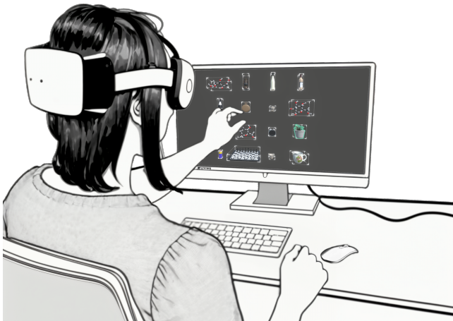
Figure 3: The setup for our initial study. The participants sat in front of a monitor wearing an HMD. A grid of objects is presented in the desktop environment, and a similar grid is shown in AR next to the participants. Image transformed using Stable Diffusion.
