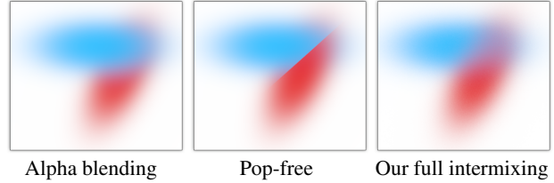
Figure 5. Fully volumetric intermixing – While alpha blending (left) suffers from popping and “pop-free” variants (middle) show discontinuities, our full volumetric intermixing (right) accurately composes overlapping Gaussians.
