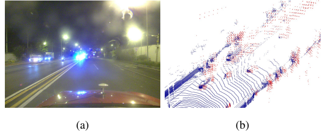
Fig. 1: Visualization of camera, LiDAR and 4D mmWave data in rainy nighttime. The raw data is from the Dual Radar dataset [13]. (a) shows the camera image. (b) illustrates LiDAR point clouds in blue and 4D mmWave radar (Arbe Phoenix) point clouds in red.
