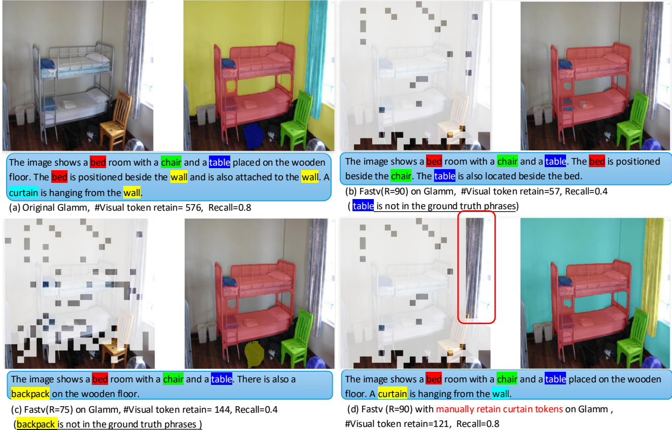
Figure 1. (a): Result of original GLaMM [22]. (b): Result of GLaMM with Fastv [4] method pruning 90% of visual token starting from the second layer. (c) : Result from GLaMM with Fastv method pruning 75% of visual tokens starting from the second layer. (d): Results from GLaMM using FastV [4] with 90% visual token pruning and retaining additional visual tokens retained at the curtain location, starting from the second layer. Comparing (c) and (d), we could conclude that “Local Information Matters” : preserving visual tokens corresponding to object locations provides richer object information to the vision-language model.
