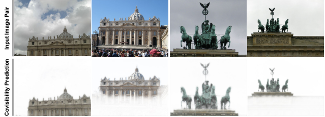
Figure 2. Visualization of covisibility prediction. We first bilinearly up-sample the covisibility score map to match the original image resolution, and then multiply it with the input image.
