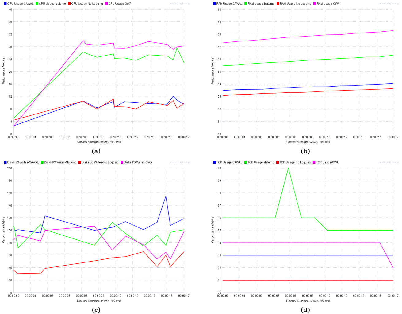
Fig. 7. Load test resource usage comparison of equivalent on-premises web analytics tools.
