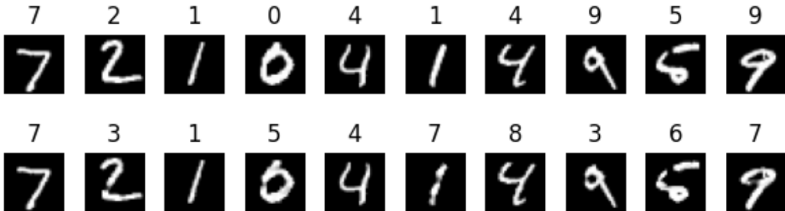
FIGURE 8. Original images (top) vs. adversarial images (bottom). The number above each image is the prediction of a tropical network with base model LeNet5.
