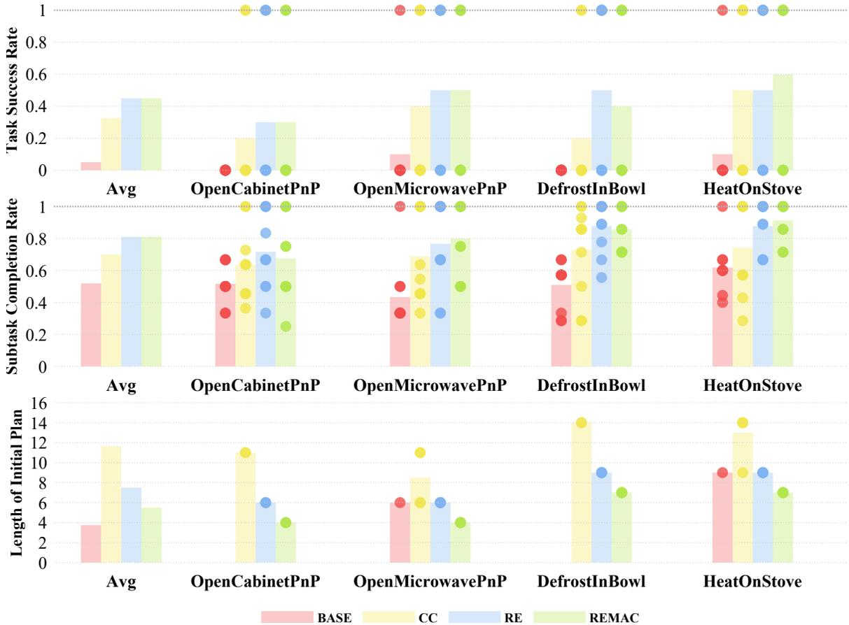
**Fig. 4:** Our experimental results indicate that: (1) condition checking and reflective evolution effectively enhance both the Task Success Rate and the Subtask Completion Rate; (2) compared to single-robot systems, multi-robot systems demonstrate a reduced Length of Initial Plan and greater efficiency. All tasks were subjected to rigorous validation through ten randomized initializations across four distinct experimental settings.
