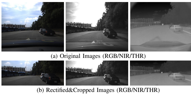
Fig. 5: Image pre-processing for MS 2 dataset. We rectified and cropped the original RGB, NIR, and thermal images with intrinsic and distortion parameters to make valid training data.
