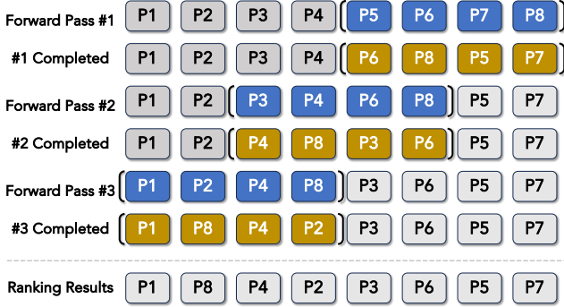
Figure 4. Illustration of sliding window re-ranking for N = 8 gallery images with a list-wise re-ranker that can re-rank K = 4 images each forward pass. Blue blocks represent the re-ranking window of the current forward pass, and it slides to the next window with a stride of S = 2 images. Brown blocks indicate the re-ranking for the current forward pass is completed.
