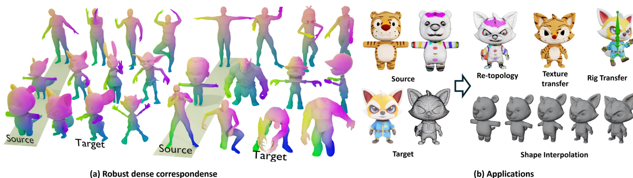
Figure 1. We propose Stable-SCore: A Stable Registration-based Framework for 3D Shape Correspondence. Given a source and a target mesh, our approach registers the source mesh to the target and establishes dense correspondence between them, with strong robustness to large variations in mesh topology, shape, and pose, as shown in (a). Our method enables a range of downstream applications, including re-topology, texture transfer, rig transfer, and shape interpolation, as shown in (b).
