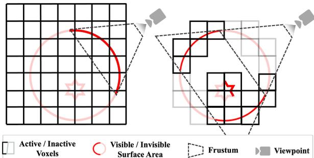
Figure 3. **Frustum-aware sectional voxel training.** The previous mesh-based rendering training strategy (left) requires activating the entire dense grid to extract the mesh surface, even though only a few voxels are necessary during rendering. In contrast, our approach (right) adaptively activates the relevant voxels and enables the reconstruction of mesh interiors only using rendering supervision.
