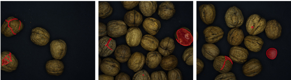
Fig. 9. Example images from the TEST_{pub} set for Walnuts . The defects depicted here are cracks, holes, and contamination by foreign bodies, in this case a hazelnut. Similar to the Wall Plugs scenario, walnuts appear in random positions and quantity. Additionally, walnuts exhibit large natural variations in their color, shape, and size. Defects occur all over the image, including close to the image borders.
