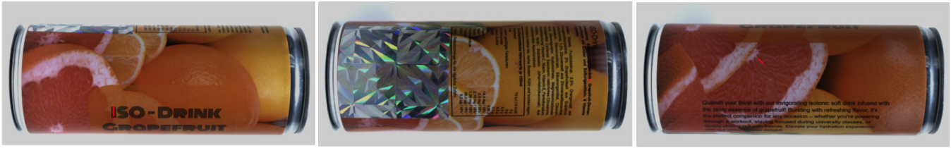
Fig. 7. Example images from the TEST_{pub} set for Can . The can is randomly rotated and contains a glitter foil to cover barcode information, which adds additional allowable variation. The defects depicted here are print errors, changes in color, and scratches. Other defects include missing can labels.
