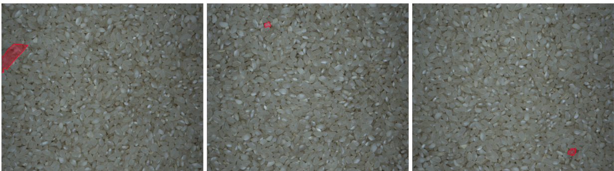
Fig. 12. Example images from the TEST_{pub} set for Rice . The defects depicted here are plastic foil and foreign bodies that were chosen to be visually similar to rice in shape, size, and color. Other defects include hairs. Defects occur all over the image, including close to the image borders.
