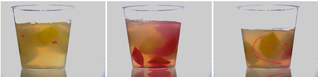
Fig. 11. Example images from the TEST_{pub} set for Fruit Jelly . The defects depicted here are alien objects like metal flakes and vegetable pieces as well as hairs. Other defects include further types of contaminations or scratches in the glass. For completeness sake, the reflection of the defects on the bottom of the setup were labeled as well. Differently colored fruits, the refractive properties of the jelly, and the random combination of ingredients lead to a large variety in the non-anomalous data.
