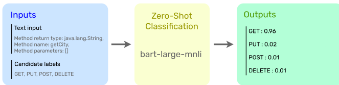
Fig. 8. Representation of the HTTP request classification process.
