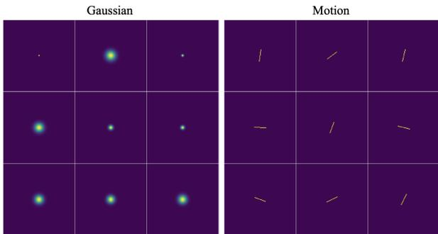
Figure 4. Ground truth point spread functions for both the Gaussian (left) and motion (right) examples.
