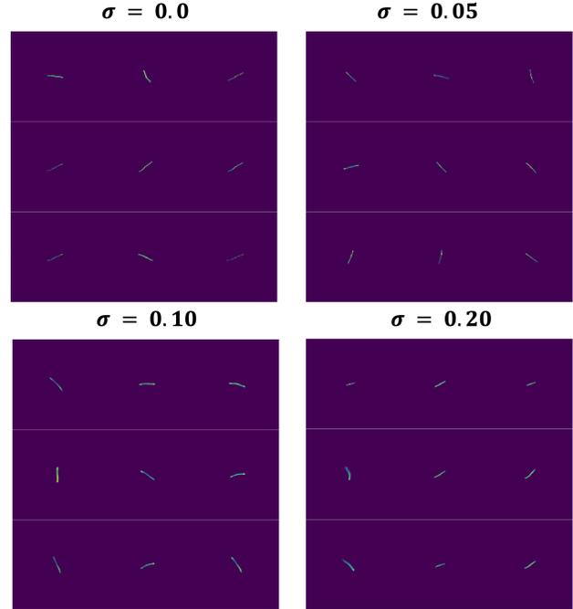
Figure 8. PSFs learned using the proposed technique on data at various noise levels.
