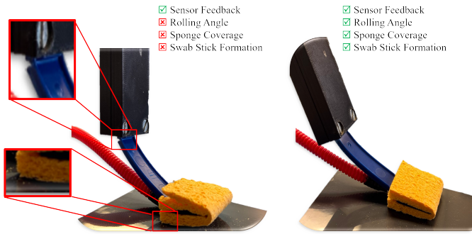
Fig. 15. Effect of Tool Distortion Due to Force Misalignment. (Left) Without the proposed algorithm, the controller compensates by increasing the rolling angle, causing excessive tool deformation. (Right) With the algorithm, force is evenly distributed, maintaining proper tool alignment and preventing distortion.
