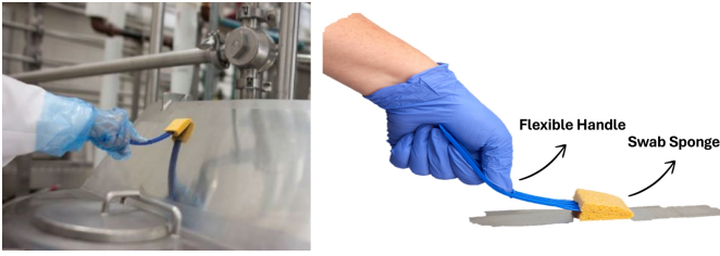
Fig. 1. Swab sampling collection model with deformable sponge stick
