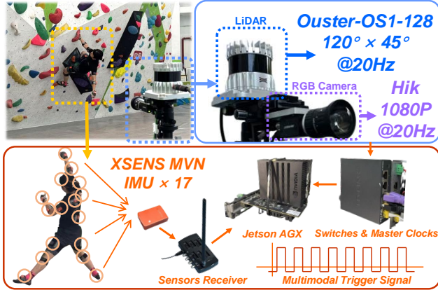
Figure 3. Dataset collection hardware system.
