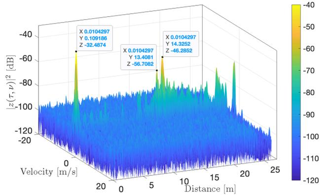
Fig. 3. Three largest peaks in 2D distance and velocity spectrum with the experiment data, obtained by (4) at the  $m$ -th RIS sweep angle corresponding to  $\phi = [0^\circ, 0^\circ]^T$ .
