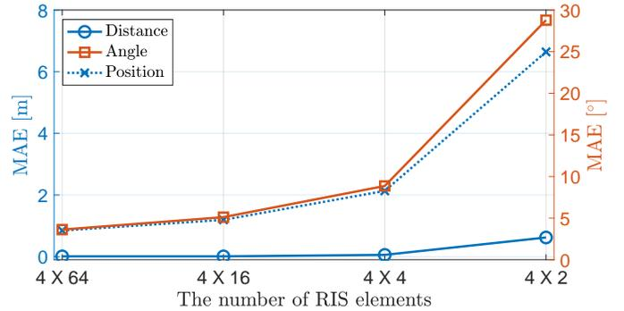
Fig. 8. MAEs of distance, angle, and position estimates with the different number of RIS elements.
