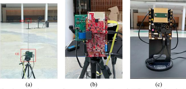
Fig. 2. Experiment environment, where UE and RIS are deployed: (a) displacement of UE and RIS; (b) UE; and (c) RIS.
