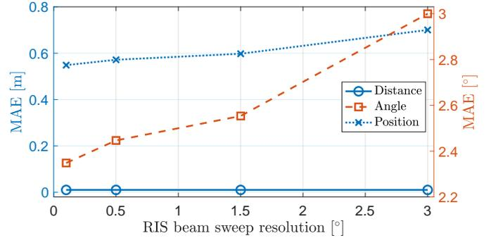
Fig. 7. MAEs of distance, angle, and position estimates with the different RIS beam sweep resolutions.
