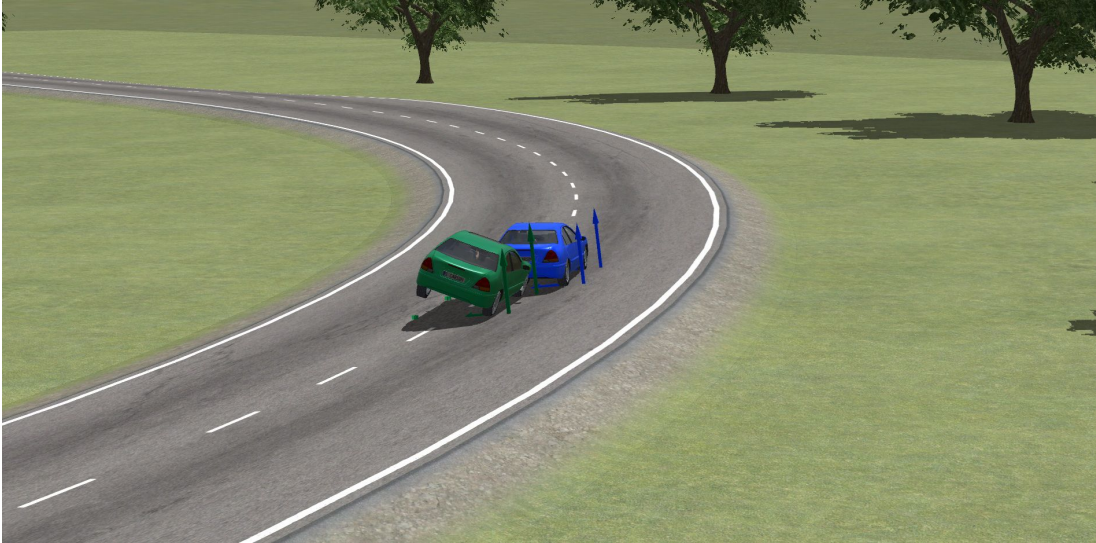
Fig. 5: A snapshot of the CarSim environment illustrating the implementation of DeePC1 and LMPC1. The image captures the moment at t = 21.7s , where the green vehicle (LMPC1) violates the LTR constraint and begins to lose stability, while the blue vehicle (DeePC1) successfully navigates the sharp turn.
