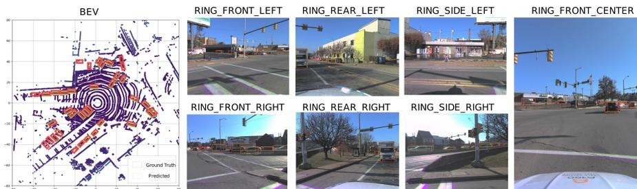
Fig. 5: A qualitative comparison of long-range 3D object detection using multi-modal fusion methods on AV2-C validation set. BEV maps on left, 2D image space on right. Red: Ground truth, Green: Predicted boxes.
